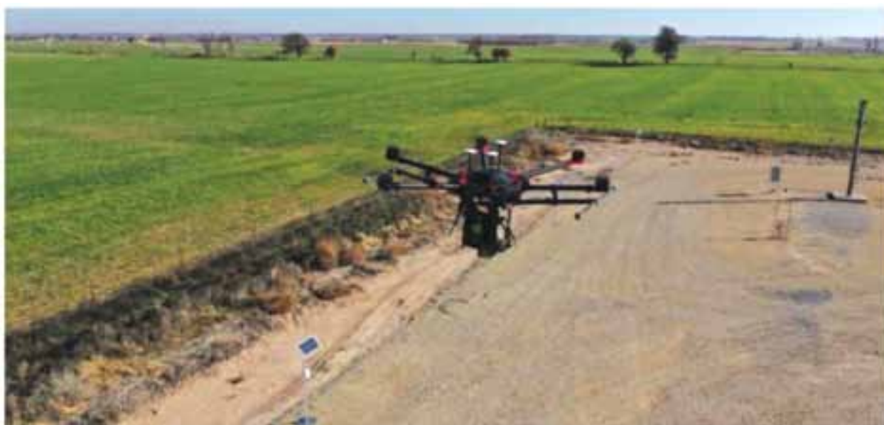
Figure 6—Using drones to detect methane leaks (Jacobs 2019 / Baker Hughes)
